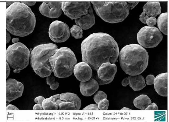
cross section and topography after milling in the Nara Hybridizer (NH) for 4 min, 16000 rpm
